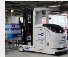
Autonomous forklift Receiving, dispatching
